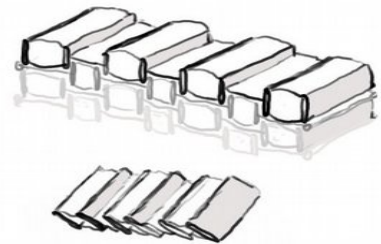
Picture 6.59: Multi-chamber bags with firming supporters: up—unfolded, down—folded.
