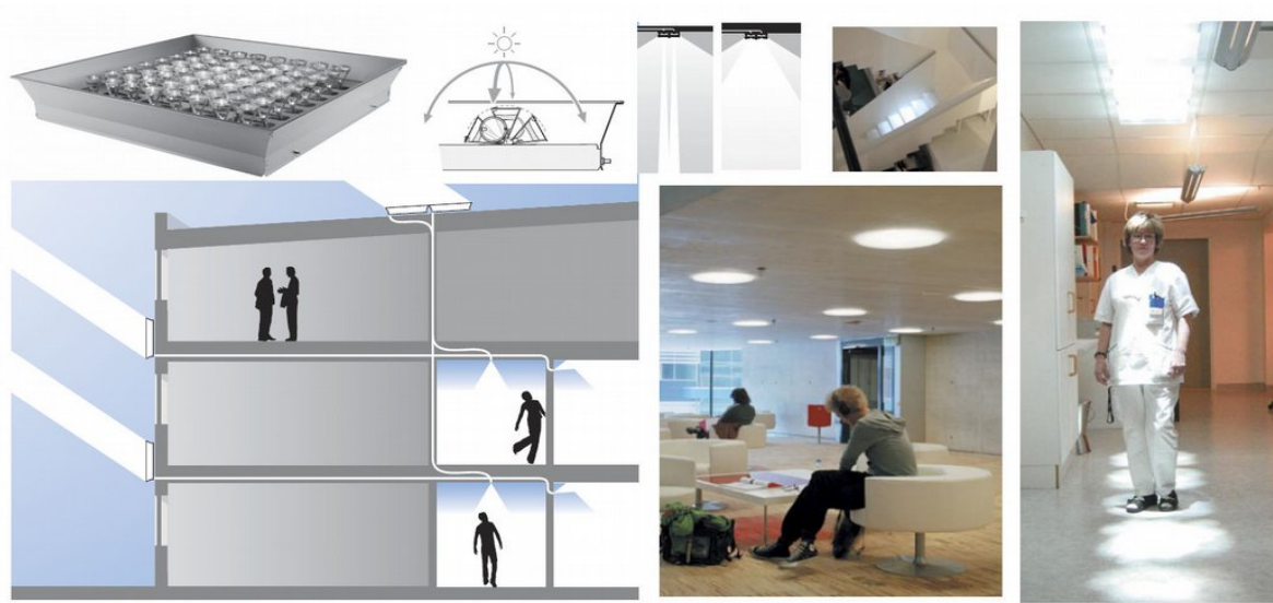
Picture 6.117: Parans Daylighting System for transportation of concentrated Sun-light via optical fibers to the emitters inside (Parans Daylight AB)
