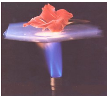
Picture 6.65: Aerogel is a very good thermal isolator (JPL/NASA)
